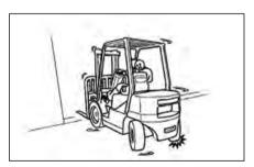
An unloaded forklift may be easier to tip over than a loaded truck.
