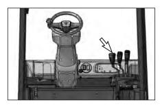
The forks' lift control is located at the operator's right side front. The lift control lever is the lever at the left.
