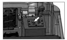
Loosen the bolts of the hydraulic tank top plate assembly.
