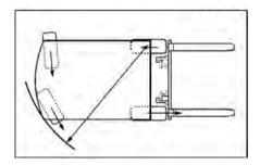
As the steer wheel angle increases, the inside drive motor speed is progressively slowed down with respect to the outside drive motor speed.
