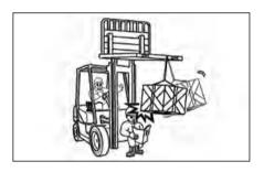
Carrying a load suspended on a chain or a cable may unbalance a truck.
