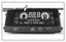
14. Check the LCD display for battery discharge status. A fully charged battery will be displayed on the LCD display.
