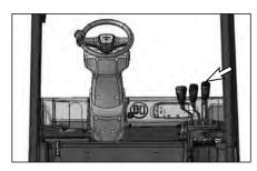
The sideshift attachment control is located at the operator's right side front. The sideshift attachment control lever is the lever at the right.
