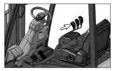
To slow, stop or change direction when traveling in either direction, move the the directional control forward/reverse switch (1) to the opposite direction while keeping the accelerator pedal (2) depressed.
