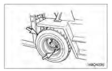
Inspect tires and valve stems for wear, cuts, gouges and foreign objects.
