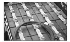
Check the specific gravity of the battery. If the specific gravity reading is below 1.150, the battery must be charged.
