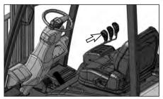
Move the directional control forward/reverse switch into NEUTRAL.
