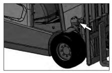
8. Inspect the hydraulic system for leaks, worn hoses or damaged lines.
