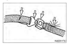
If the seat belt is torn, if pulling motion is interrupted during extension of the belt, or if the belt cannot be inserted into the buckle properly, replace the seat belt assembly.
