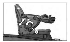
Turn No. 2 knob leftwards (CCW) to adjust the arm rest position up/down.
