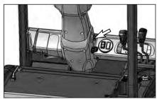
Turn the key switch to the ON position. Raise the attachments.
