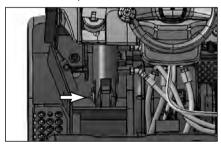
Lubricate pivot eyebolts, one fitting on each tilt cylinder.
