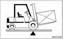
Counterbalanced lift truck design is based on the balance of two weights on opposite sides of a fulcrum (the front axle). The load on the forks must be balanced by the weight of the lift truck.
