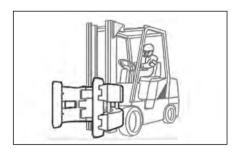
There are many special attachments available to replace the forks on a lift truck.
