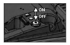
**Parking brake activation** - The parking brake is automatically engaged with a "clunk" after the vehicle stops.
