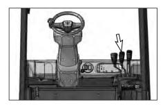
The forks' tilt control is located at the operator's right side front. The tilt control lever is the lever at the center.
