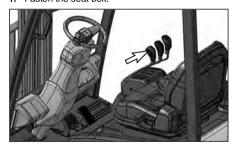
Move the directional control forward/reverse switch into the NEUTRAL position, if it is not already in this position.
