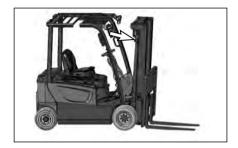
4. Tilt the mast forward and lower forks to the floor.
