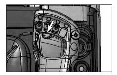
The auto tilt controller is at the rear side of the tilt knob. Press the auto tilt switch to turn on the switch lamp and push the tile knob forward. The mast will stop at 90 degrees angle.
