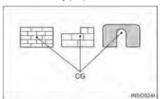
The point within an object, at which the whole weight of the object may be regarded as being concentrated, is called the center of gravity or CG. If the object is uniform, its geometric center will coincide with its CG. If it is not uniform, the CG could be at a point outside of the object. When the lift truck picks up a load, the truck and load have a new combined CG.
