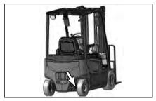
Lubricate fitting on steer axle.
