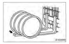
Block drums or round objects. Tilt mast forward and slide fork tips along the floor to get under the load.
