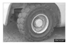
Install the steer wheel. Put two nuts opposite each other (180°). Tighten both. Install all remaining nuts. Tighten all nuts in a crisscross sequence opposite each other (180°) to a torque of 113 N·m (85 lb·ft).
