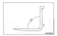
Check the angle between the upper face of the blade and the front face of the shank. The fork should be withdrawn from service if angle (C) exceeds 93 degrees or deviates by more than 3 degrees from an original angle other than 90 degrees, as may be found in some special application forks.
