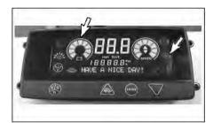
Check the indicator LCD display for the discharge state of the battery and the brake oil level.
