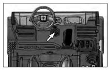
5. To stop the lift truck where conditions do not permit electrical braking(plugging). Release the accelerator pedal (1). Push down on the service brake pedal (2) and bring the lift truck to a smooth stop.
