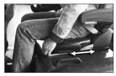
Use the lever at the left-hand side to adjust the seat to the position you desire.
