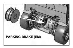
**3.** The parking brake is automatically engaged with a "clunk" after the vehicle stops.
