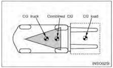
The stability of the lift truck is determined by the location of its CG; or, if the truck is loaded, the combined CG of the truck and load. The lift truck has moving parts and, therefore, has a CG that moves. The CG moves forward or backward as the mast is tilted forward or backward. The CG moves up or down as the mast moves up or down. The CG and, therefore, the stability of the loaded lift truck, are affected by a number of factors such as:
