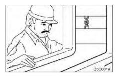
Establish a daily and 12 month inspection routine by keeping a record for the forks on each lift truck.
