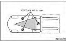
For the lift truck to be stable (not tip over forward or to the side), the CG must stay within the area of the lift truck stability base – a triangular area between the front wheels and the pivot of the steer wheels. If the CG moves forward of the front axle, the lift truck will tip forward. If the CG moves outside of the line on either side of the stability base, the lift truck will tip to the side.
