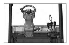
The auto tilt controller is on the left side of the tilt knob. Press the auto tilt switch to turn on the switch lamp and push the tile knob forward. The mast will stop at 90 degrees angle.
