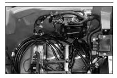
Clean the control panel with 205 kPa (30 psi) maximum air pressure, until dust is removed from the control panel.
