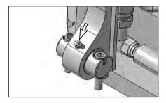
2. Lubricate the mast hinge pins. One fitting on each side of the mast. Total of two fittings.
