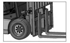
Inspect tires for wear, cuts, gouges and foreign objects. Look for bent rims and correct seating of locking ring.
