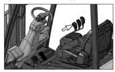
Move the directional control forward/reverse switch to the opposite direction of lift truck travel.
