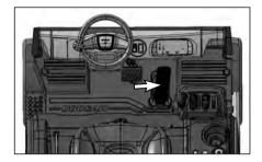
**Accelerator Pedal -** The accelerator pedal is located on the floor of the operator's compartment.
