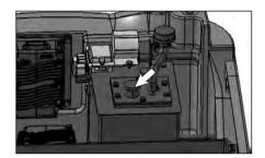
3. Remove an discard the hydraulic filter.
