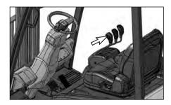
17. With the seat switch closed and the directional control forward/reverse switch in NEUTRAL, turn the key switch ON. Observe the battery discharge indicator.
