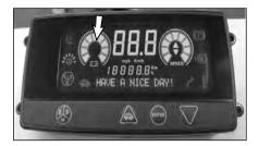
18. Make sure the battery is charged before operating the lift truck. A fully charged battery will cause "9 Segments" to be displayed on the BDI display.
