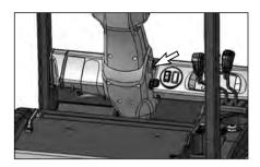
The key switch is located on the right side of the steering column.
