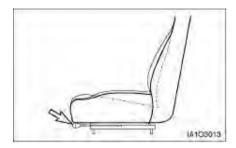
15. Position the seat by operating the lever and moving the seat forward or backward to a comfortable position
