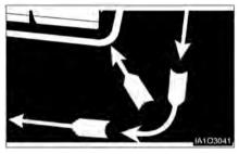
When turning in narrow aisles, keep as far from the stockpile as possible when making a turn into the aisle. Allow for counterweight swing.
