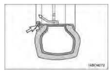
Do NOT inflate a tire that has been run while flat or underinflated, without first checking to make sure the locking ring on the wheel is not damaged and is in position.
