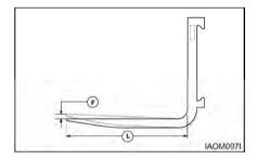
4. Check the difference in height of one fork tip to the other when mounted on the fork carrier. A difference in fork tip height can result in uneven support of the load and cause problems with entering loads.
