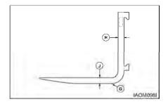
Check the fork blade (J) and shank (H) for wear with special attention to the heel (G). The fork should be withdrawn from service if the thickness is reduced to 90 percent or less of the original thickness.
