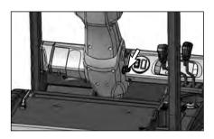
11. Adjust the steering wheel to a comfortable position.
