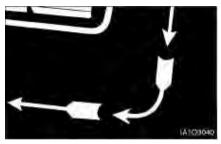
When turning sharp corners, keep close to the inside corner. Begin the turn when the inside drive wheel meets the corner.
