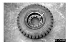
Remove the wheel assembly. Examine the wheel for damage and wear. Replace the wheel if necessary.
