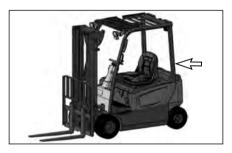
Inspect the overhead guard for damage, loose or missing mounting bolts.
