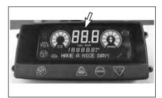
If the warning is ignored, lift interrupt will prevent the hydraulic pump motor from operating and an "EL" will be displayed on the LCD display.
