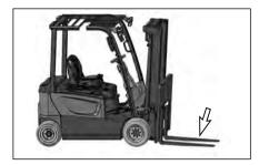
1. Lower the forks and tilt the mast forward.
