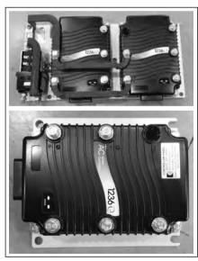
4. Inspect all wiring for loose connections, frayed cables and loose mounting bolts.
