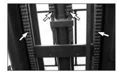
**6.** Inspect the chain anchors and individual links for wear, loose pins or cracked leaves.
