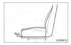
Move the lever to adjust the seat forward or backward. Release the lever. Move the seat slightly to lock it.
