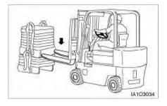
2. Move the lift truck forward until the load touches the carriage
