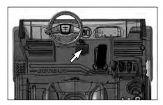
**Service Brake -** The service brake pedal is located on the floor of the operator's compartment.
