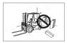
Do not operate forklifts near flammable o combustible materials.
