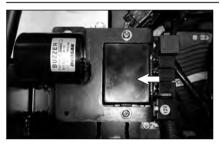
Backup & Stop Lamp - 5 A ISO Relay & POWER -5A FAN & FINGERTIP -5A Rear Lamp - 5 A Strobe & Flasher -5A DC-DC & Horn - 20 A – 5A R Head Lamp Lamp (OPT) -5A Kev Switch - 10 A L Head Lamp - 5A
