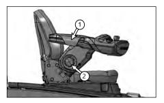
Using the two adjustment device, adjust the positions of the arm rests to a comfortable positions.
