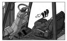
12. Move the directional control forward/reverse switch to NEUTRAL.
